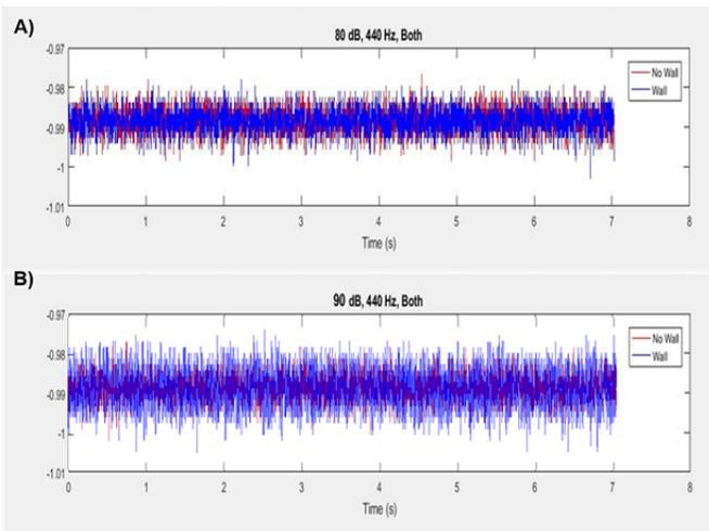
Fig. 8. Vibration induced at (A) 440 Hz (80 dB) and (B) 48.1 Hz (90 dB) when display case is freestanding or mounted to wall. A composite plot is depicted to compare the normalized acceleration. [Freestanding: Red and Mount to Wall: Blue].
