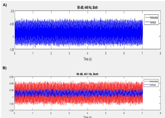
Fig. 6. Vibration induced at (A) 440 Hz (98 dB) and (B) 48.1 Hz (96 dB) in the horizontal and vertical Komatex display block orientation. A composite plot is depicted to compare the normalized acceleration. [Horizontal: Red and Vertical: Blue].
