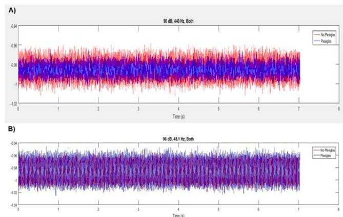
Fig. 5. Vibration induced at (A) 440 Hz (90 dB) and (B) 48.1 Hz (96 dB) in the absence and presence of Plexiglas cover. A composite plot is depicted to compare the normalized acceleration. [No Plexiglas: Red and Plexiglas: Blue].
