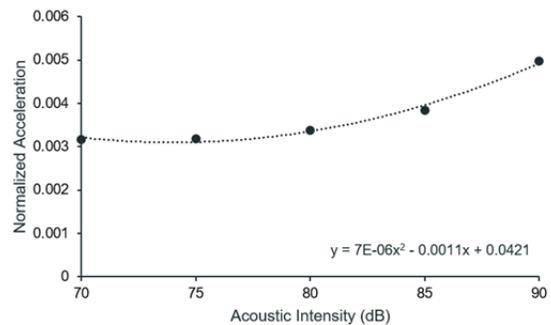
Fig. 4. Normalized acceleration plot depicting the relationship between the music intensity and the vibration induced.
