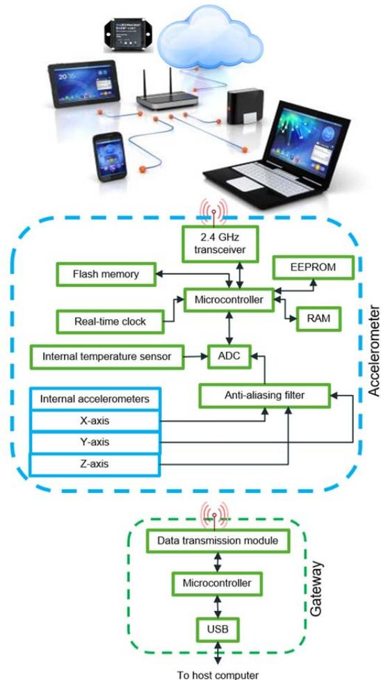
Fig. 2. Diagram of accelerometer and gateway system architecture.
