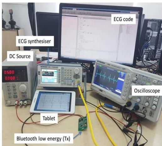
Fig. 4. Real time experimental setup for demonstration.
