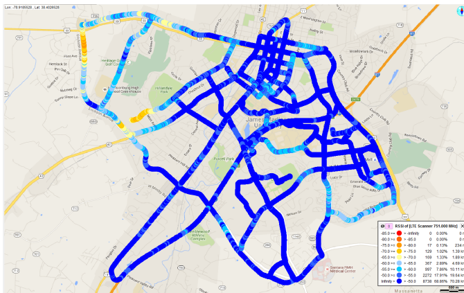
Fig. 6. The RSSI of 751 MHz in the downtown area of the authors' city using the Anritsu Linkmaster system.
