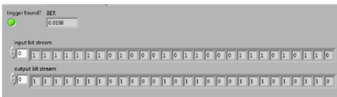
Fig. 5. LabVIEW front panel of the Input/output bit stream & BER.
