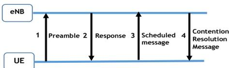
Fig. 4. NB-IoT RACH 4-steps procedure.
