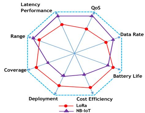
Fig. 5. NB-IoT & LoRa: IoT factors based comparison.
