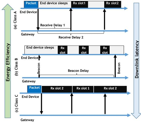
Fig. 3. Three classes device receive slot timing.
