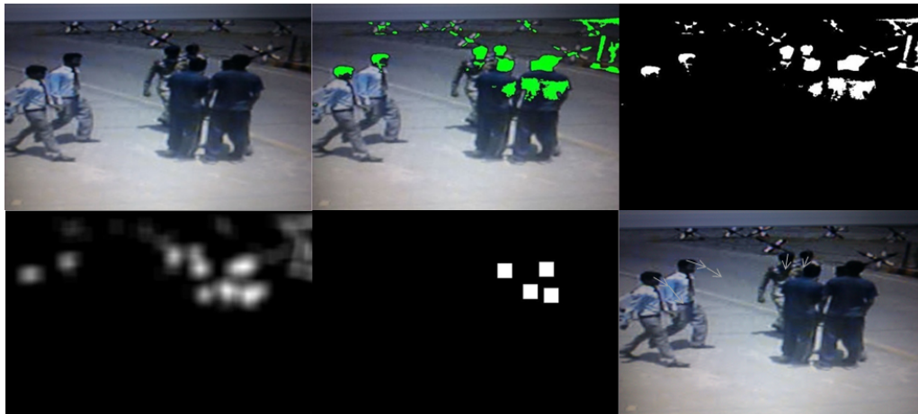
Fig. 3. (a) Original Frame showing abnormal behavior, people approaching a reference point (b) Heads Identification (c) Binarization using Adaptive thresholding (d) Correlation with previous frame (e) Head Detection (f) Inward direction on the bases of Motion Vectors.
