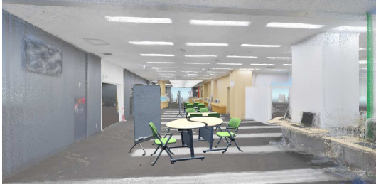
Fig. 11. Replacement of ArUco codes with 3D models.
