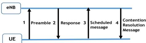
Fig. 4. NB-IoT RACH 4-steps procedure.
