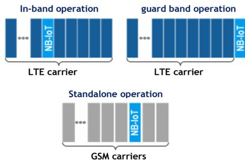
Fig. 2. NB-IoT band operational modes.
