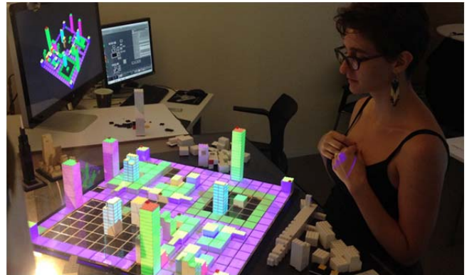
Fig. 3. Demonstrative system with illuminated tangible interactive matrix and 3D projection mapping.
