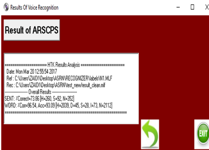
Fig. 6. Automatic recognition system result of continuous pathological speech (ARSCPS) with ETSI FE V2.0 (MFCC_0_D_A).
