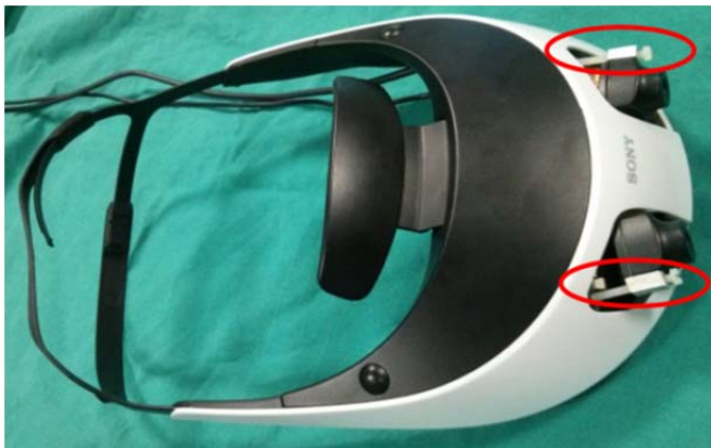
Fig. 4. HMD prototype embedded with adjuster screws for stereo camera vergence control.
