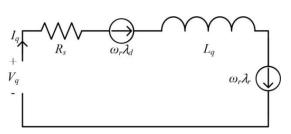
Fig. 6. Dynamic Model of PMSM in Q axis.
