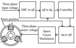
Fig. 4. General Block Diagram of FOC.
