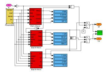
Fig. 3. Model Scheme of the Centrifugal Pump.
