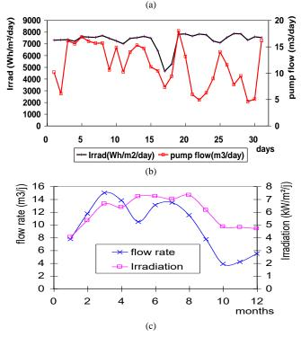
Fig. 11. Experimental Results of the PV Pumping Systems: Hourly Variations (a), Daily Variations (b) and Monthly Variations (c) of the Pump Flow and the Irradiance
