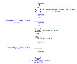
Fig. 2. ETAP Modeling of the Induction Furnace.
