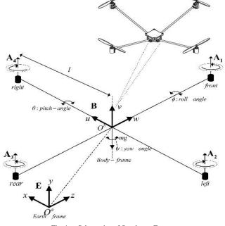
Fig. 1. Schematics of Quadrotor Forces.
