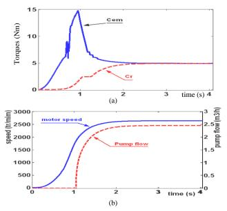
Fig. 7. (a): The Electromagnetic and Resistant Torques, (b):The Motor Speed and Pump Flow.
