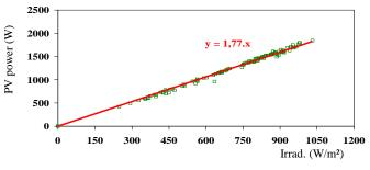
Fig. 13. Variation of the PV Power versus the Irradiance.
