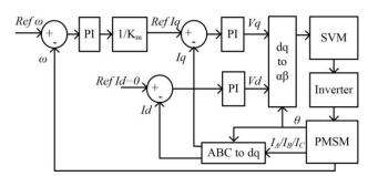
Fig. 7. Speed Control of PMSM by FOC.
