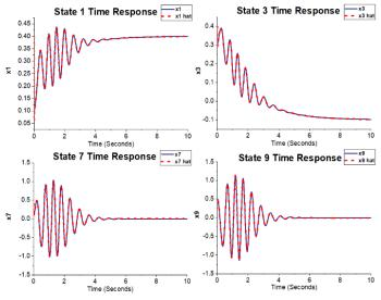
Fig. 3. State 1, 3, 7, 9 and Estimated State Trajectory of Quadrotor.
