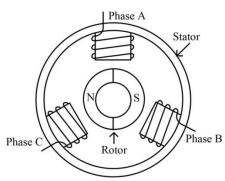
Fig. 1. Basic Structure of PMSM.
