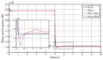
Fig. 8. PI Controller Robustness under L<sub>s</sub> Variations.
