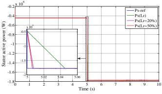
Fig. 11. Sliding Mode Controller Robustness under Lr Variations.
