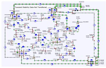
Fig. 5. The IEEE 37 Bus 9 Generators Test System.
