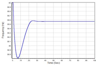
Fig. 6. The Frequency of the System when the PEAR138 Generator Disconnects.
