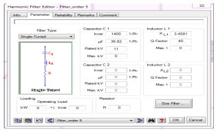
Fig. 13. Modeling Passive Filters (Single Tuned Filter).
