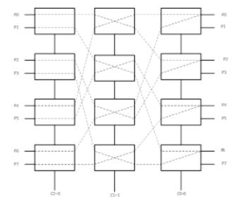
Fig. 9. The Reconfigurable Architecture with Eight Nodes.
