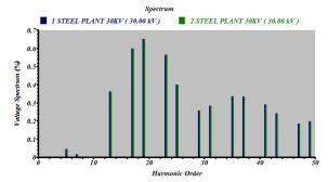
Fig. 19. Voltage Spectrum at Steel Plant 30KV Bus with Filters.
