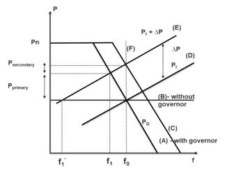
Fig. 4. The Relationship between Frequency Deviation and Output Power Deviation.
