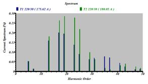
Fig. 21. Current Spectrum at Al-Taba Transformer 220/30KV with Filters.
