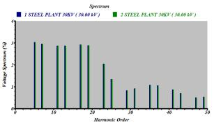
Fig. 8. Voltage Spectrum at Steel Plant 30KV Bus.
