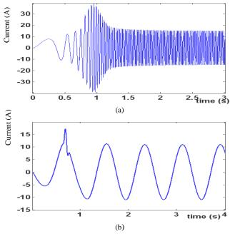
Fig. 6. Variation of the Stator (a) and Rotor (b)Currents.
