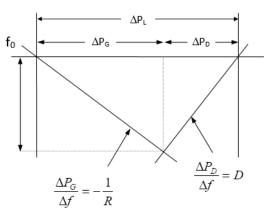
Fig. 3. Synthesized Frequency Response of the Power System.
