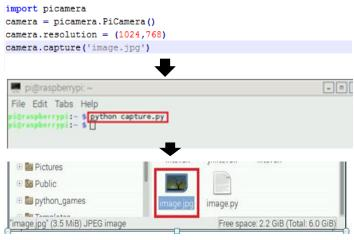
Fig. 8. Camera Functionality Test.
