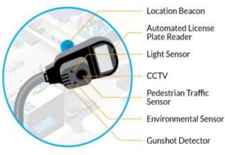
Fig. 4. Sensors Housing in Smart Street Light Poles [6].
