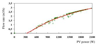
Fig. 14. Variation of the Pump Flow versus the PV Power.
