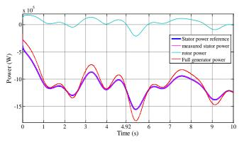
Fig. 15. Power Balance and Tracking Response of Stator Active Power.
