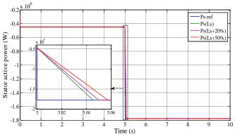
Fig. 9. Sliding Mode Controller Robustness under Ls Variations.
