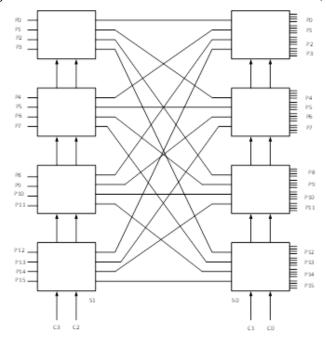
Fig. 8. The Reconfigurable Architecture with 16 Nodes.
