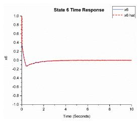
Fig. 7. State 6 and Estimated State Trajectory of Quadrotor.
