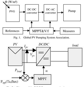
Fig. 2. Diagram of the DC-DC converter monitoring strategy
