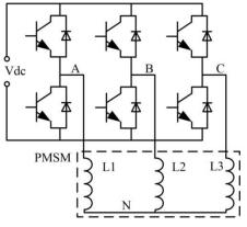
Fig. 2. Three Phase Invertor Circuit for PMSM.
