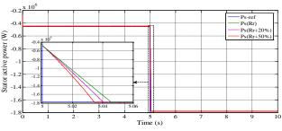
Fig. 7. Sliding Mode Controller Robustness under Rr Variations.
