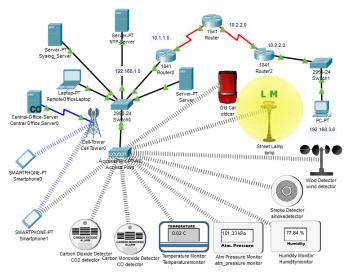
Fig. 6. Model Simulation Design for Different Sensors.
