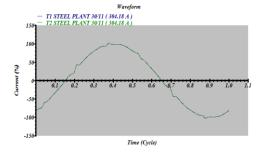
Fig. 24. Current Waveform at Steel Plant Transformer 30/11KV with Filters.
