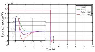
Fig. 6. PI Controller Robustness under R<sub>r</sub> Variations.
