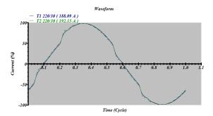
Fig. 9. Waveform for the Current at Al-Taba Transformer 220/30KV.
