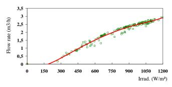
Fig. 12. Variation of the Pump Flow versus the Solar Radiation.
