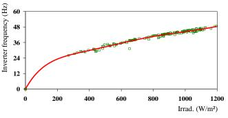
Fig. 15. The Inverter Frequency versus the Solar Radiation.
