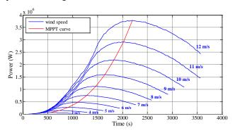
Fig. 3. Optimal Power Curve for Different Wind Speeds.
