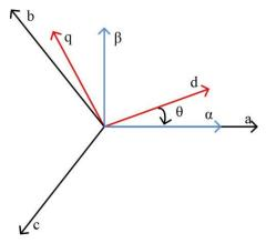
Fig. 3. Two and Three Phase Reference Systems.
