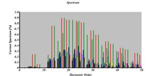
Fig. 23. Current Spectrums at All Transformer 30/11KV with Filters.
