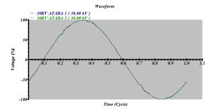
Fig. 16. Voltage Waveform at Al-Taba 30KV Bus with Filters.
