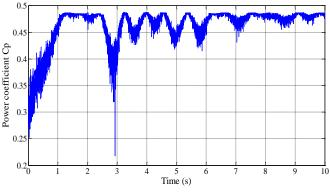
Fig. 14. Ppower Coefficient Cp using OP-MPPT.
