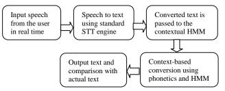
Fig. 1. Architecture of Proposed Phonetic Model.
