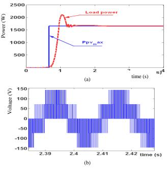
Fig. 5. (a): Adaptation of the Load Power to the Maximum PV Generator (b): Output Inverter Voltage.
