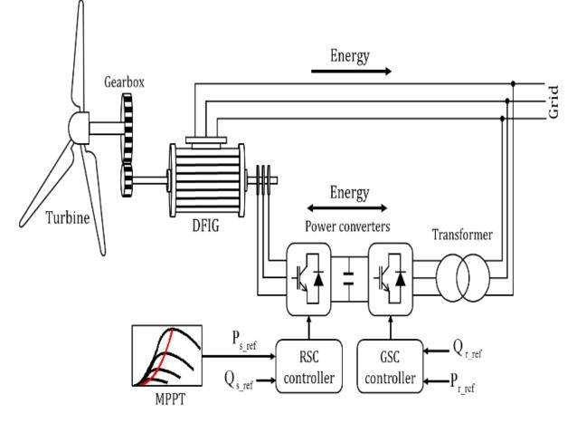
Fig. 1. Architecture of DFIG based wind System.
