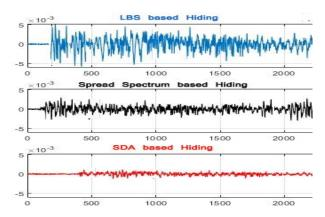
Fig. 28. Waveform differences between the Original Audio Streams and the Watermarked Audio Streams in the Three Approaches under the Gaussian Noise Attack.
