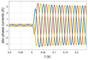
Fig. 16. Three Phase Currents While Load Torque Changes.
