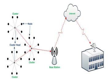
Fig. 1. A Typical Wireless Sensor Network with clusters
