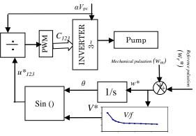
Fig. 4. Synoptic of the Three-Phase Inverter V/f Law.
