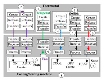
Fig. 5. The TM Representation of the Thermostat.
