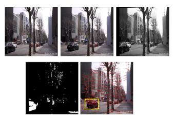
Fig. 6. Moving object detection after motion compensation. (a) frame  $(I_{t-1})$  (b) frame  $(I_t)$  (c) the warped frame using the homography matrix H calculated based on the optical flow from the two consecutive frames (d) the thresholding result for frame subtraction (c - b) (e) the final output where moving object with maximum area is detected, red arrows show the optical flow results for the detected points.
