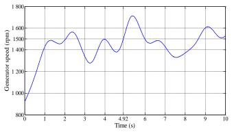
Fig. 13. Mechanical Speed of DFIG Shaft.
