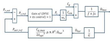
Fig. 4. OP-MPPT Control Structure.
