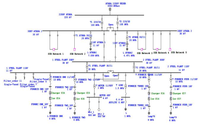
Fig. 1. Overall One Line Diagram Grid Presentation.
