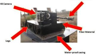
Fig. 4. Proposed Sewerbot with all Components.
