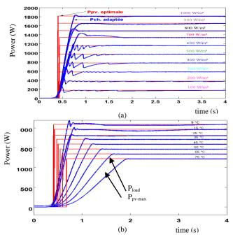
Fig. 8. Power Adaptation: (a): Several Irradiance and 25°C, (b) Several Ambient Temperature and 1000W/m<sup>2</sup>.
