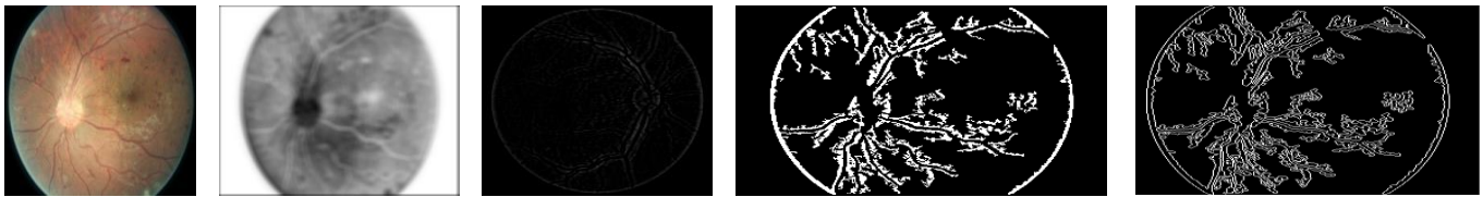
Fig. 3. Segmentation Results of the Proposed Method based on SVD and Morphological Opening on Retinal Images:(a) Depicts the Input Retinal Images with Blood Vessels, (b) Shows the Contrast Enhancement Image using SVD, (c) Depicts the Subtracted Image of Gray and Average Filter, (d) and (e) Shows the Final Blood Vessels Segmentation and its Perimeter of the Resultant Image Respectively.
