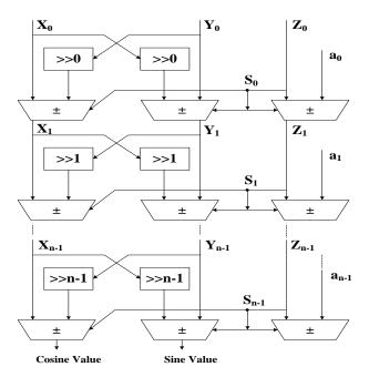
Fig. 3. Pipelined Structure used in Optimized CORDIC Model..
