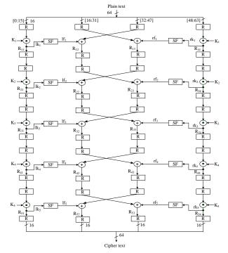
Fig. 3. Architecture of Encryption Module.
