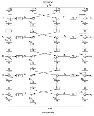
Fig. 4. Architecture of Decryption Module.
