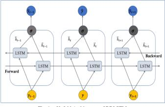
Fig. 1. Unfold Architecture of BDLSTM.
