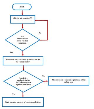
Fig. 3. PbPc Array Algorithm for NO<sub>2</sub> Detection.
