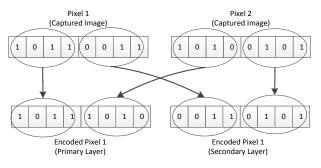
Fig. 5. Encoding Captured Image Pixels into Two Layers
