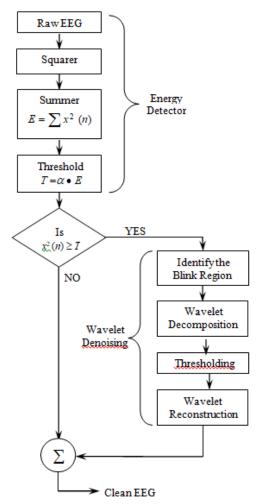
Fig. 1. Flow Chart for Detection and Correction of Blink Artifacts.
