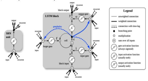
Fig. 7. LSTM Recurrent Neural Network.
