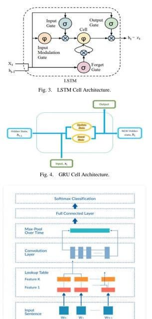
Fig. 5. CNN Architecture for Text Classification [12].
