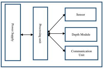
Fig. 1. Internal Architecture of underwater Node.
