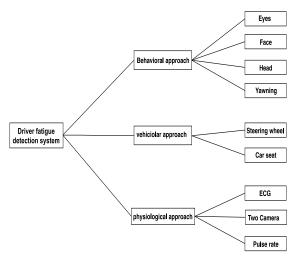
Fig. 1. A Visual Example of Driver Fatigue Detection (DDD) Systems based on different Apporaches.
