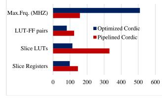
Fig. 8. Resource Comparison of Both Pipelined and Optimized CORDIC Models.
