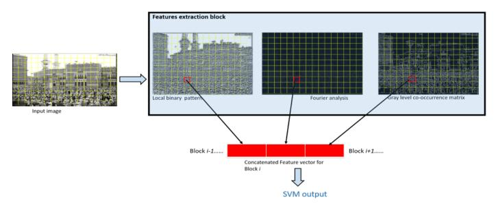
Fig. 2. Sample input frame is divided into multiple blocks. Feature are extracted for block *i*(red). Features are concatenated and feed to the SVM classifier to assign a score.
