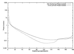
Fig. 6. A Comparison of Phase Functions between Aerosol and Cloud Particles Calculated with Mie Scattering Theory.
