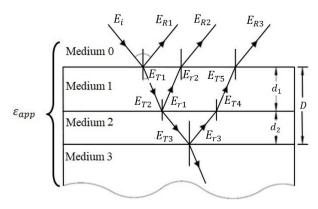
Fig. 1. Multilayered Soil Reflection Model [8].
