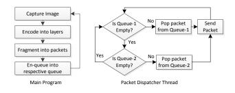
Fig. 4. Processes running on camera node
