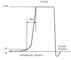
Fig. 5. The Definition of Slope Factor (D99).
