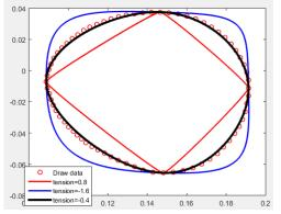
Fig. 12. Interpolation Curvers from 4 Key Points with different Tension Parameters.
