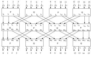
Fig. 2. Architecture of S-BOX Function (SF).
