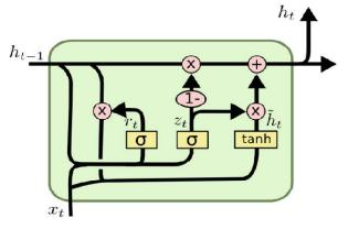
Fig. 2. A typical GRU Block Diagram.
