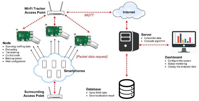
Fig. 1. Wi-Fi Tracker System Architecture.
