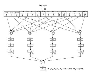
Fig. 1. Architecture of Key Generation Module.
