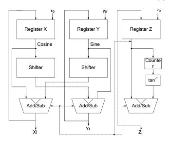
Fig. 1. Hardware Architecture of the Pipelined CORDIC Model.
