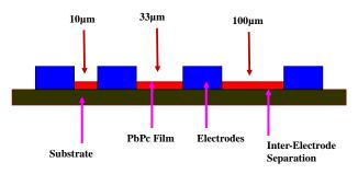
Fig. 2. Cross Section of the used PbPc Chemiresistor Array.
