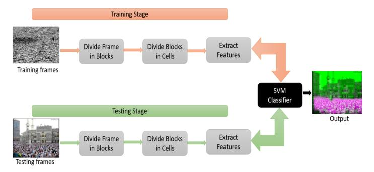
Fig. 1. Pipeline of proposed framework both during testing and training phase. Input image is divided into block and the into cells. Features are then extracted from each cell and train SVM classifier.
