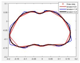
Fig. 13. Interpolation Curves from 12 Key Points with different Tension Parameters.
