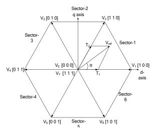
Fig. 2. Fundamental Sectors and Switching Vectors.
