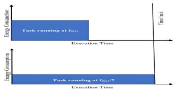
Fig. 1. Dynamic Voltage Frequency Scaling.
