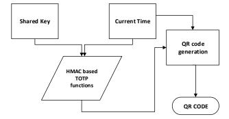
Fig. 2. TOTP based QR Generation Procedure Flow Diagram.
