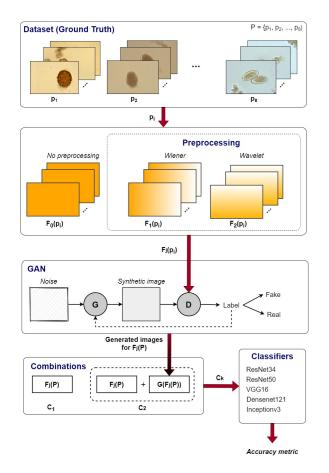
Fig. 1. Methodology. Top images should correspond to a specific species of parasite; then, it could be applied filter wiener or wavelet denoising as a preprocessing technique. After this, a DCGAN is able to generate images with one generator and one discriminator. Finally, ground truth and generated images are evaluated with classifiers Resnet34, Resnet50, and VGG. The process of data augmentation is applied independently for each parasite species.
