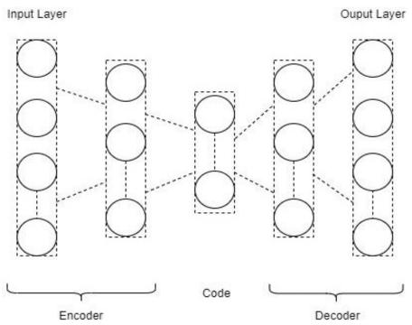
Fig. 1. An Autoencoder Structure.
