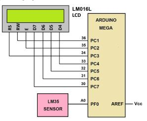
Fig. 1. Circuit Example based on the Arduino Mega.
