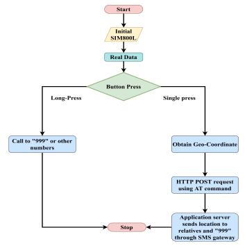
Fig. 1. The Working Framework for our Anti-Molestation Safety Device. Here, "999" is the Bangladeshi Emergency Telephone Number, and the "AT" Denotes the Attention Command to Send Location via Geo-Coordinate.
