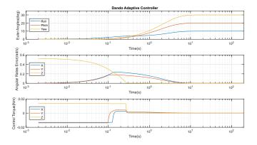
Fig. 11. Euler Angles, Angular Rate Errors and Control Torque produced by the Dando Adaptive Controller defined in (41) and (45) with a settling time (ts) of 6.33 s and average computational cost (O) of 0.200 ms. The Control Torque saturation time was 267 ms.
