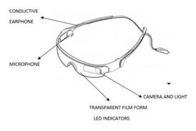
Fig. 3. Design of the Electronic Glasses
