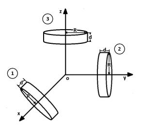
Fig. 1. Distribution of the reaction wheels described in the body frame which origin coincides with the center of mass and geometric. The loads are considered to be fully balanced around the 'o' origin. Adapted from [2].
