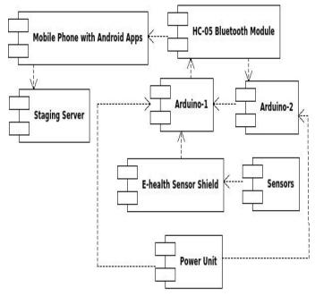
Fig. 6. Physical Arrangements of the Components of the Developed Toolkit.
