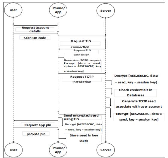
Fig. 3. A High-Level Diagram of TOTP Enrolment Process.
