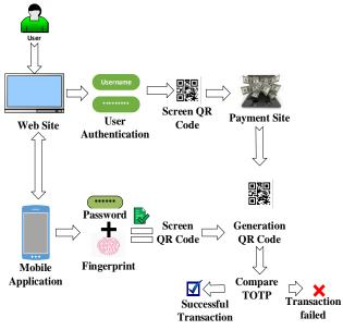
Fig. 6. Proposed System Architecture.
