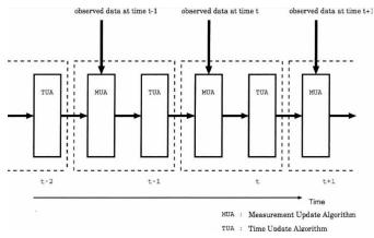
Fig. 2. Kalman Filter Consists of the Measurement Update Algorithm [Equation (5), (6), and (7)] and the Time Update Algorithm [Equation (3), and (4)].
