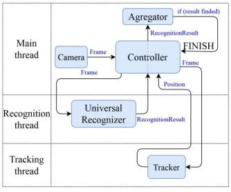
Fig. 2. Distributed Recognition Module Architecture.
