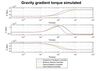
Fig. 13. Gravity gradient torque disturbance for a 100 Km low orbit CubeSat.
