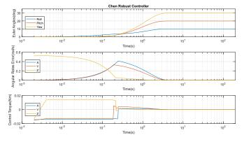
Fig. 12. Euler Angles, Angular Rate Errors, and Control Torque produced by the Chen Robust Controller defined in (52) with a settling time (ts) of 2.75 s and an average computational cost (O) of 0.309 ms. The Control Torque saturation time was 235 ms.
