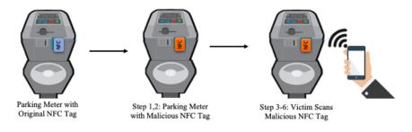
Fig. 3. Phishing Attack Targeting at Parking Meter
