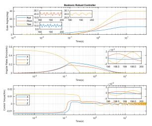
Fig. 5. Euler Angles and Angular Rate Errors produced by the miscellaneous disturbance torque in the Controller defined in (33) with a settling time (ts) of 6.44,  $\pm$  0.04 degrees in the Euler Angles oscillations,  $\pm$  1.8 ×10<sup>-3</sup> rad/s oscillations in angular rates, and  $\pm 2.1 \times 10^{-3}$  Nm in Control Torque.
