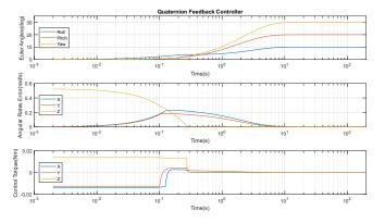
Fig. 9. Euler Angles, Angular Rate Errors and Control Torque produced by the Quaternion Feedback Controller defined in (27) with a settling time (ts) of 6.83 s and Average Computational Cost (O) of 0.027 ms. The Control Torque saturation time was 267.5 ms.
