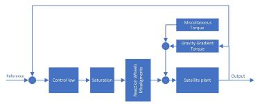
Fig. 3. Block diagram for a CubeSat subject to gravity gradient torque, and misalignment. The control law block may have adaptation algorithms depending on the simulated control law.
