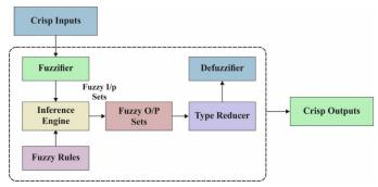
Fig. 2. Block Diagram of T2FL.
