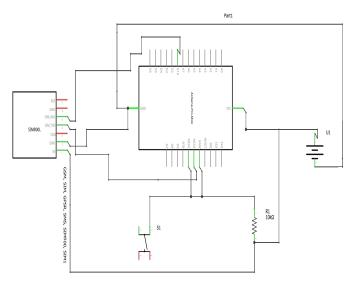
Fig. 4. The Circuit Diagram of the Device. Here, S1, R1, and U1 denotes the Switch, Resistance and Battery, Individually.
