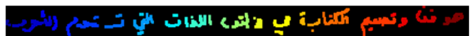
Fig. 6. Shape Segmentation based on 8 Neighbour Connected Pixels (Colors are only used to Illustrate Different Objects)
