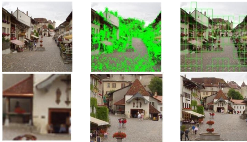
Fig. 2. First Row Detected SURF Local Features (Middle), Selected Blocks (Right), Second Row (Left) Sample Selected Block (Level 0), Level 1 Patch (Middle), Level 2 Patch (Right).
