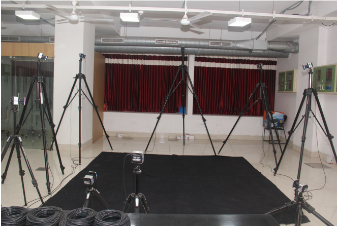
Fig. 1. 3D motion capture system for hand gesture capture
