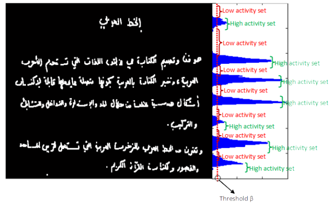
Fig. 5. Define High and Low Activity Sets based on Histogram of Image Lines (Horizontal Lines)
