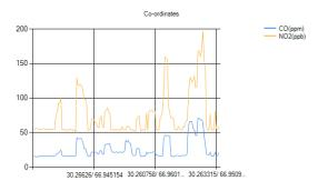
Fig. 5. CO & NO2 Values Verses GPS Co-Ordinates, Measured by Hardware Deployed in Vehicles.
