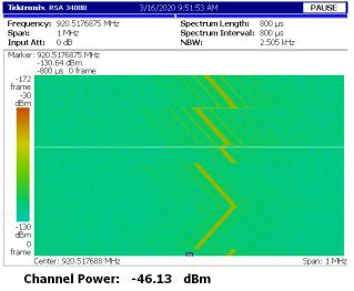
Density: -102.15 dBm/Hz Channel Bandwidth: 400 kHz Fig. 15. Chirps LoRa 920LR.
