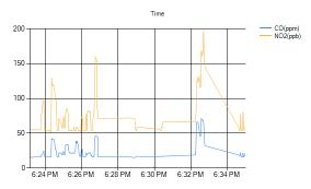
Fig. 4. Concentration Level Graph of CO (ppm) & NO2 (ppb) Verse Time, Measured by Hardware Deployed in Vehicles.
