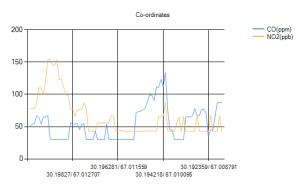
Fig. 14. CO & NO2 Values Verses GPS Coordinates, Measured by Hardware Deployed in Vehicles.
