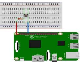
Fig. 4. Circuit Diagram for Push-Button Setup.
