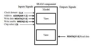
Fig. 2. The Characteristics of the SRAM Model.
