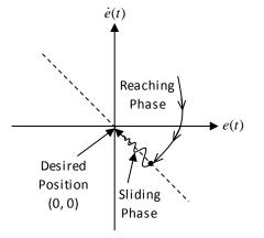
Fig 4. The Common Route to Obtain Desired Condition in SMC.
