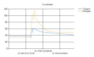
Fig. 11. CO & NO2 Values Verses GPS Co-Ordinates, Measured by Hardware Deployed in Vehicles.
