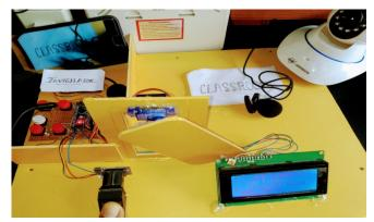
Fig 17. Opening Door Shows Successful Authentication.
