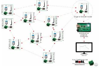
Fig. 9. Mesh Communication of Leafony board LoRa.
