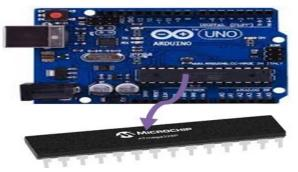
Fig 5. Arduino Uno with ATmega328P Microcontroller.
