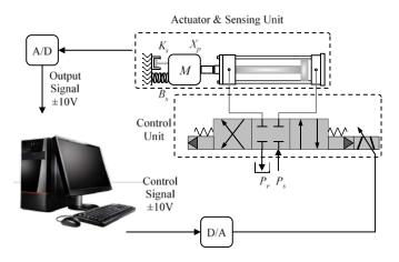
Fig 1. General Component in the EHA System.
