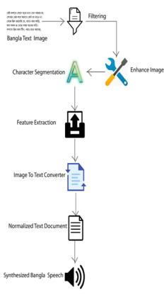
Fig. 6. System Operational Architecture.
