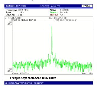
Fig. 16. Frequency Carrier of LoRa 920.592 MHz.
