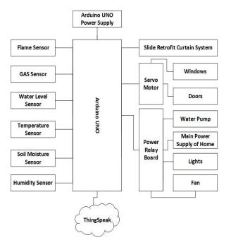
Fig. 4. Proposed Design for Arduino.
