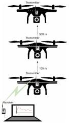
Fig. 13. LoRa Drone on FSPL Test.
