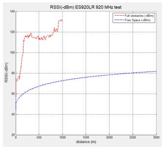
Fig. 20. FSPL and Obstacle (-dBm) RSSI Comparison.
