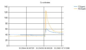
Fig. 8. CO & NO2 Values Verses GPS Co-Ordinates, Measured by Hardware Deployed in Vehicles.
