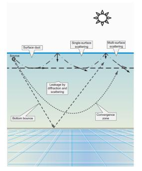
Fig. 3. Acoustic Signal Reflection and Bending Formation from [1]
