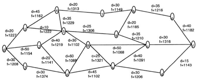
Fig. 3. The Distance (d) and Accumulated Load (f) Between Nodes Over 2000 Time Slots for 16 Nodes of Network Configuration.
