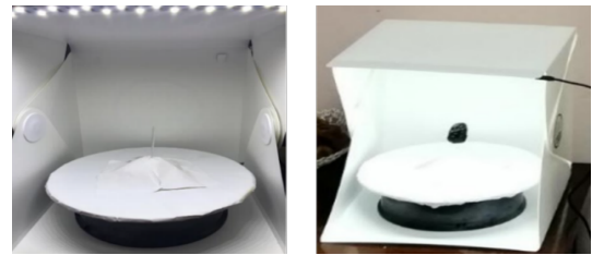
Fig. 3. The Lighted White-Compartment and the Rotating Dish used to Capture the Dataset
