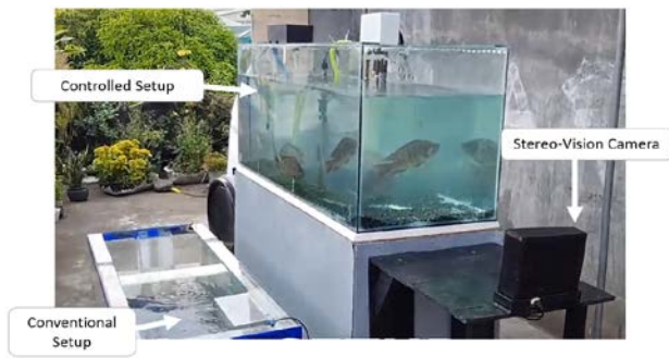
Fig. 3. Conventional and Automated Aquaculture System.
