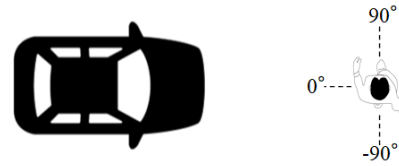
Fig. 5. Definition of the Head Pose Angle (the Geometric Relation between the Car and the Pedestrian).
