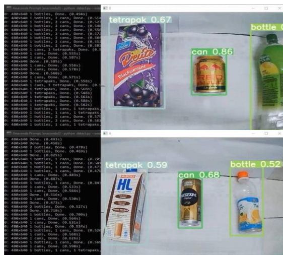
Fig. 18. Result after the Detection Module has been Tested under Condition of more than Two Classes in one Frame.
