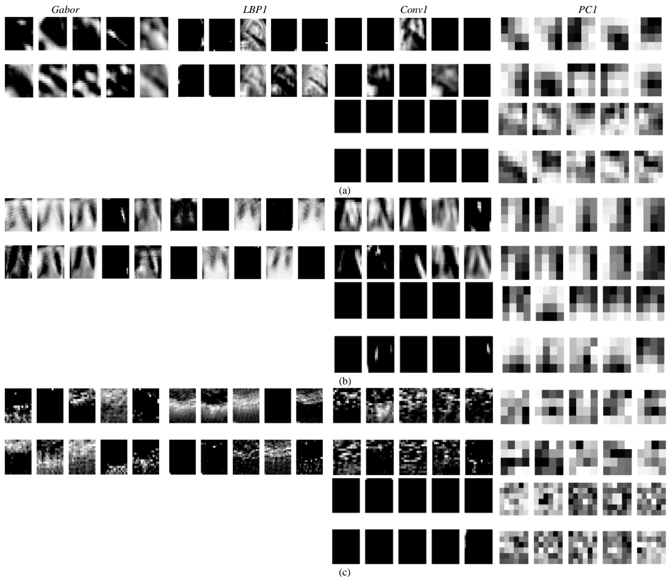
Fig. 5. Comparison of the Activation Maps of the Proposed GLC and the DR Models. (a) the First and Second Rows Show the Activation Maps for GLC and DR respectively on KVASIR, (b) Row One Shows the Activation Maps of GLC while Row Two Shows the Activation Maps of the DR Model for COVID-19, and (c) First and Second Rows are respectively the Activation Maps of GLC and DR Models for ROCT Dataset.
