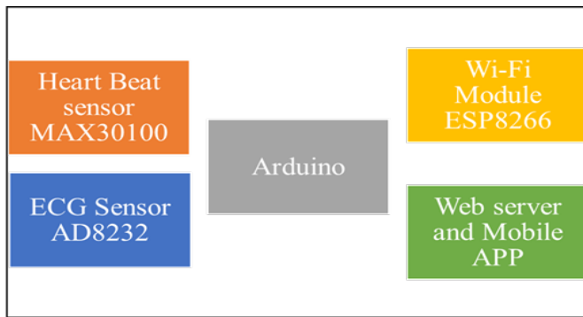
Fig. 2. Design of the IoT Device-based ECG System.
