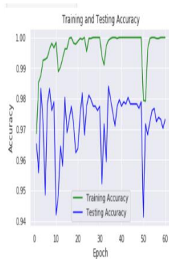
Fig. 32. Training and Testing Accuracy for ConvNet using Learning Rate of 0.00001 with 10 Disease Classes.
