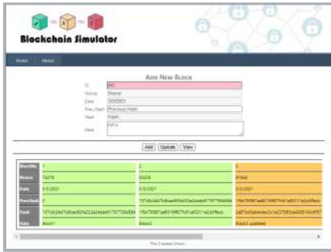
Fig. 5. Error appeared in Block 3 and the following after Modifying the Data in this Block during the Test.
