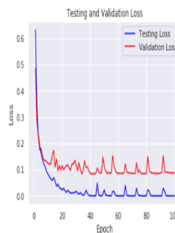
Fig. 47. Training and Testing Loss for CNN using Learning Rate of 0.001 with 16 Disease Classes.
