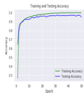
Fig. 38. Training and Testing Accuracy for CNN using Learning Rate of 0.0001 with 16 Disease Classes.
