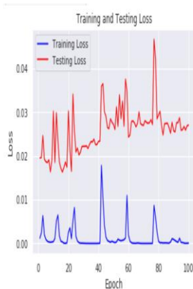
Fig. 45. Training and Testing Loss for ConvNet using Learning Rate of 0.00001 with 16 Disease Classes.
