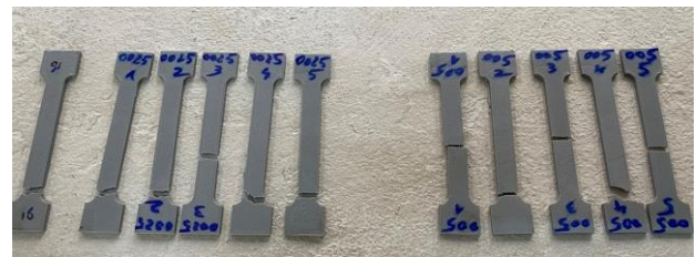
Fig. 7. Tested Samples after Traction.
