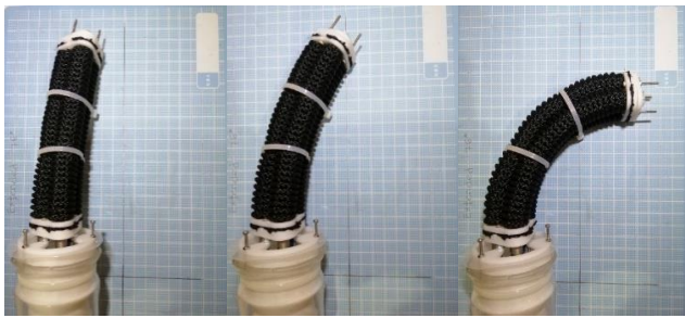
Fig. 8. View of the Curving Movement using a Bending Unit.
