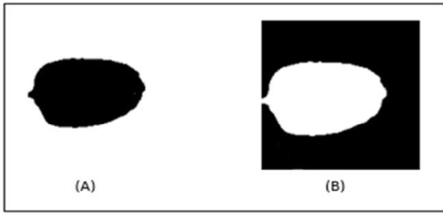
Fig. 5. Image Complement of Input Images. (A) Image after Applying Area Opening Process. (B) Image after the Complement Process.
