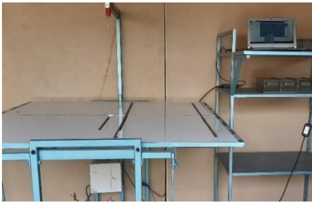
Fig. 12. Implementation of the Hot Wire Cutting Machine.
