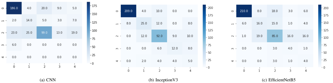
Fig. 10. The Confusion Matrix when Evaluating on the Test Set (440 Samples) for the Models Trained using the Augmented Balanced Dataset. The x-Axis Represents the Actual Labels, while the y-Axis Represents Predicted Labels. Label 0: no_DR, Label 1: mild NPDR, Label 2: Moderate NPDR, Label 3: Severe NPDR, and Label 4: PDR.
