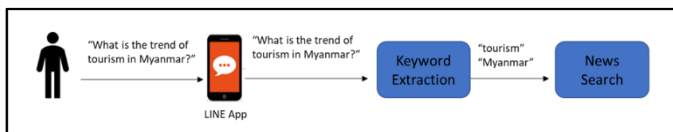
Fig. 3. An Overview of the Input and Output of the Keyword Extraction Module.
