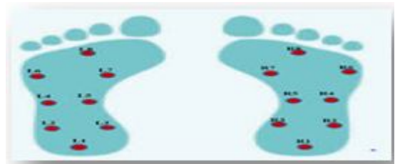
Fig. 3. Pressure Sensors Positioned under each Foot to get the Best Collection.
