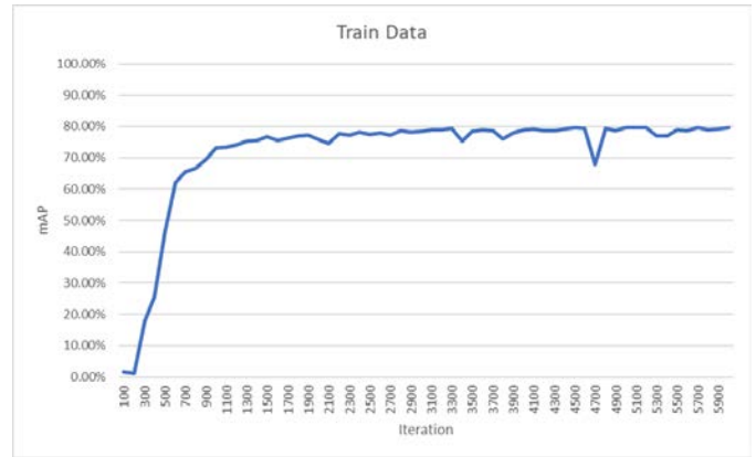
Fig. 13. Graph of Train Data Result from Split Data 70% Train, 25% Validation, and 5% Test with 0.0002 Learning Rate.
