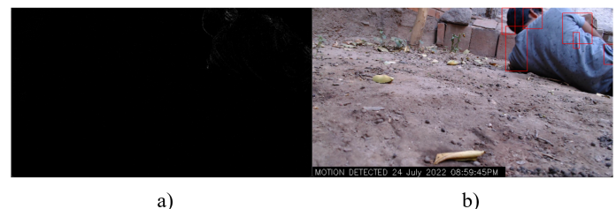
Fig. 6. Camera Frame with Detected Motion. a) Differential Window. b) Original Video Window Plus Motion Limiting Zones.
