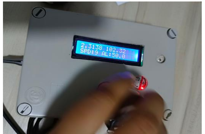
Fig. 9. Alcohol detection and location display.
