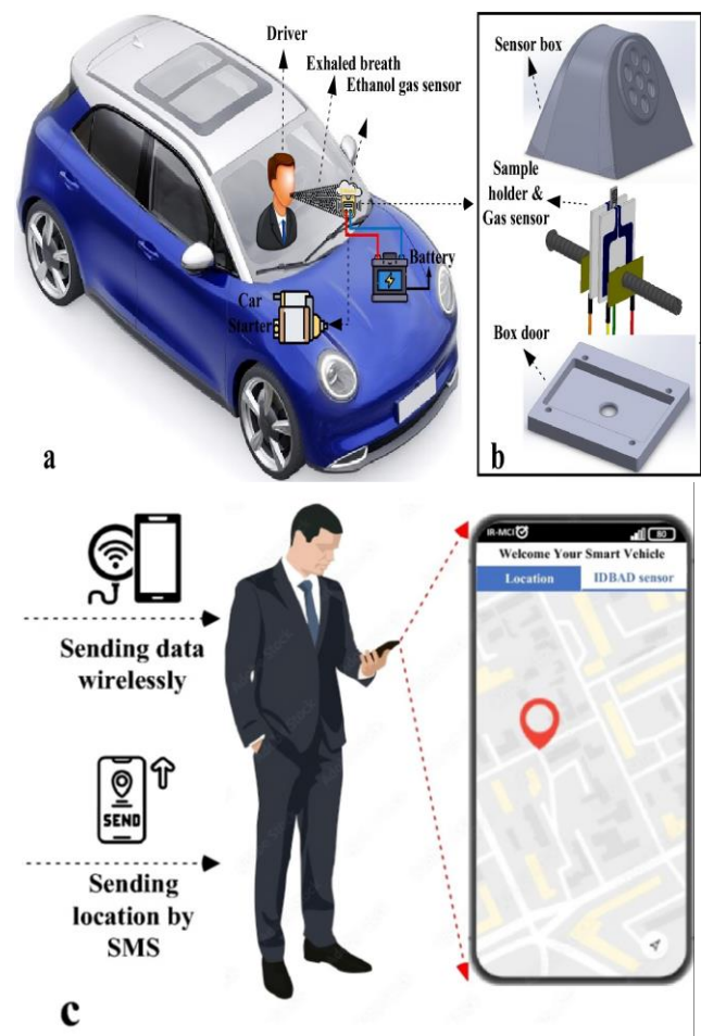
Fig. 2. Innovations in alcohol detection systems (a) Schematic and connectivity of the IDBAD system (b) Real image of the IDBAD system (c) Display information on smartphone [15].
