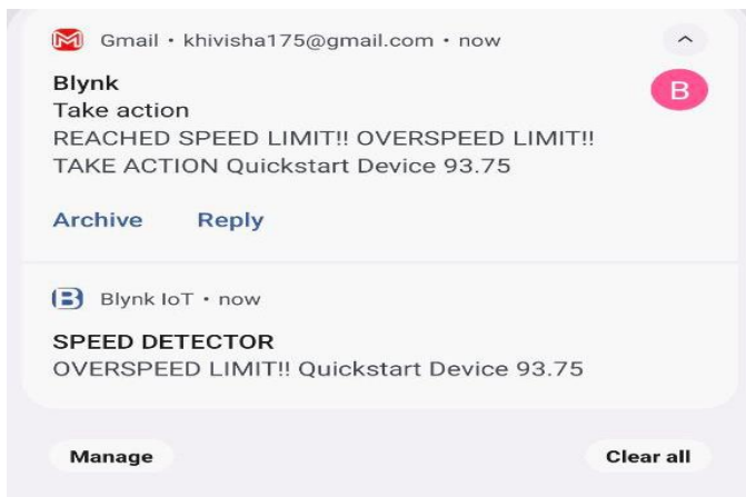
Fig. 12. Blynk notification for overspeed detection.
