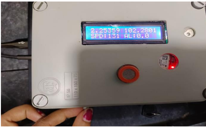
Fig. 11. Overspeed detection and location display.
