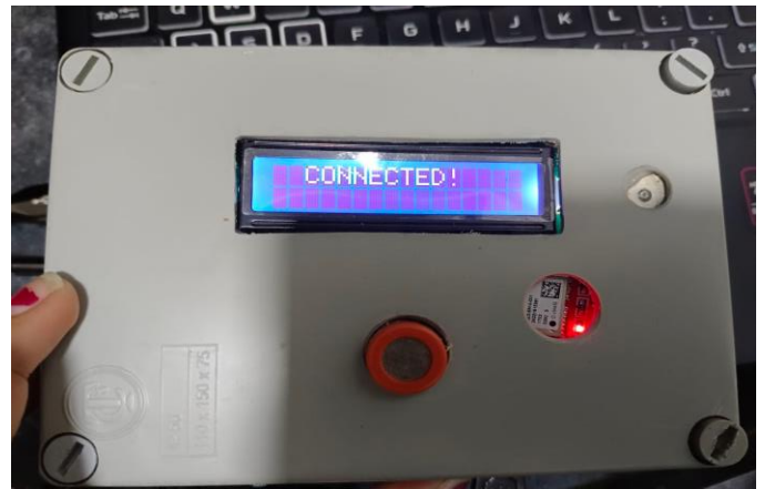
Fig. 8. Wi-Fi connection confirmation on LCD display.
