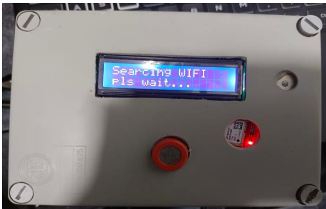
Fig. 7. Hardware initialization and connection setup.
