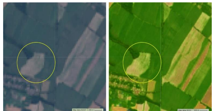
Fig. 2. RGB image 30 m (left) and the result of image sharpening through panchromatic blending, 15 m (right)
