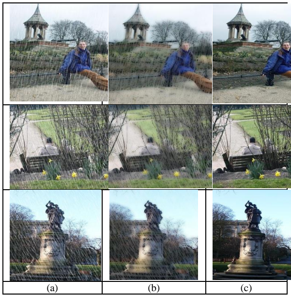
Fig. 7. Experimental outcome of Ex_GADerain: (a) Input rainy Image, (b) Detail layer extraction and (c) De-rained image
