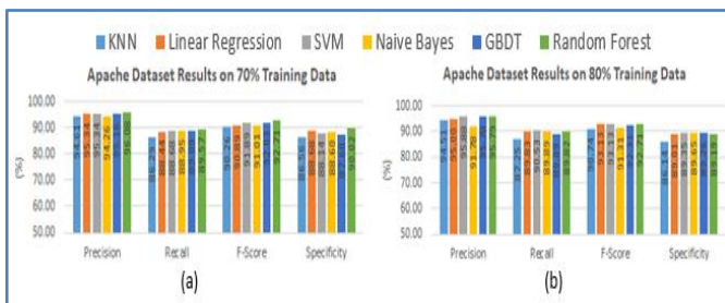
Fig. 3. Precision, recall, f1-score, and specificity in percentage on Apache datasets considering 70% and 80% of training data using BERT embedding technique.
