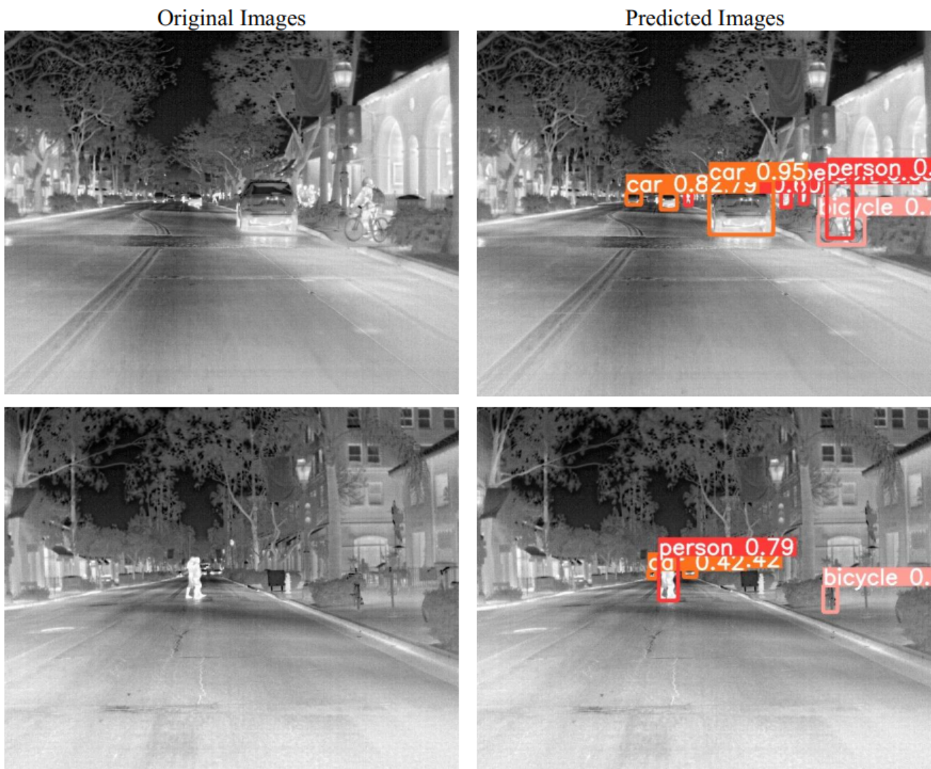
Fig. 11. Prediction results of the YOLOv5 model trained with SGD optimizer and SiLU activation function.
