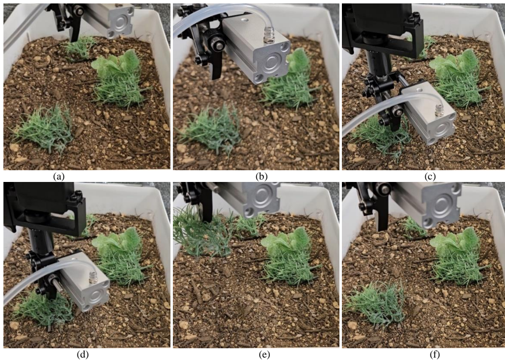
Fig. 9. Weeding Scene. (a) Initially, the robot arm is in the home position. (b) The end-effector is moved by the robot arm so that its horizontal plane coordinates match the target coordinates. (c) Based on depth information, the end-effector is lowered to the surface of the weed. (d) The end-effector grasps the weed. (e) The robot arm moves and pulls the weed out with the end-effector. (f) After releasing the grasped weed, the robot arm moves to the home position.
