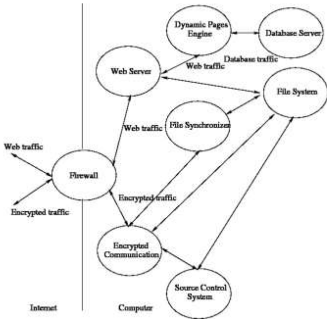
Figure 2: IT Infrastructure. We display course materials on a Web Server, and we use a Dynamic Page Engine and a Database Server to keep track of students grades. We use a File Synchronizer to maintain the same content on our desktop and laptop and we use a Source Control System to keep track of changes made to our classes. Our server is protected by a Firewall and all communication through the Internet is encrypted.
