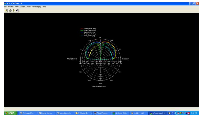
Fig. 17 Elevation Pattern of E Total, E Right, E Left, E Theta, E Phi at Phi=90 (deg)
