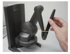
Figure 7.The haptic device, PHANTOM® DesktopTM used in the simulation system. The proximal end of the stylus is fixed with the secondary arm using a rubber band
