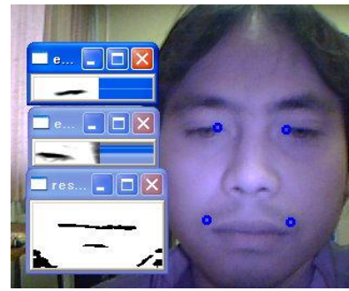
Fig.12. Face feature extracted using Gabor filter. Gabor image is shown in left side.
