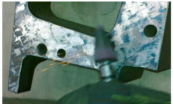
Fig.8. Removal base area – the burring
