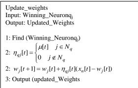
Fig. 3. b: update weights process in SOFM Algorithm
