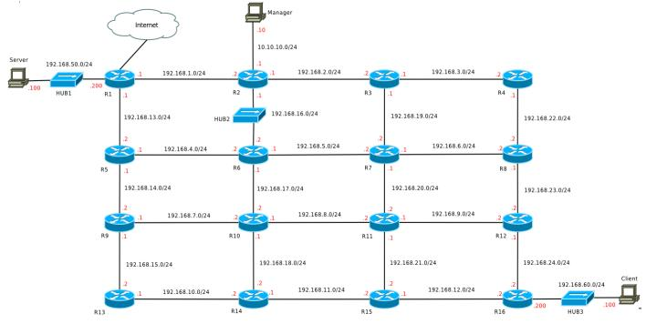
Fig. 1. Topology of the test network
