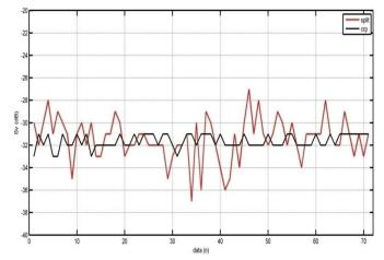
Fig. 4. Backscatter intensity of coral reef using single and split beam
