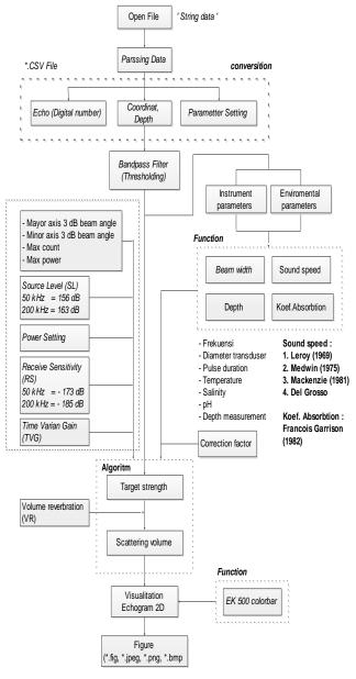
Fig. 1. Algorithm design for single beam acoustic processing
