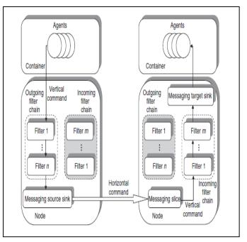
Fig. 1. Filter architecture for message kernel service [8]
