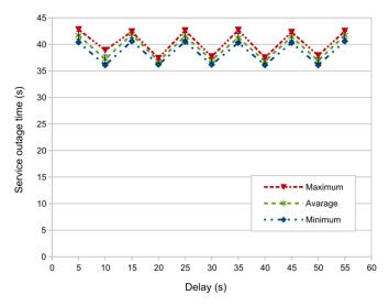
Fig. 2. Service outage times in the function of the delay from the last C-RP-Adv Message to the stopping of the R2 router
