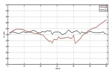
Fig. 5. Backscatter intensity of mud bottom using single and split beam
