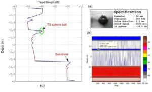
Fig. 2. Acoustic calibration using sphere ball
