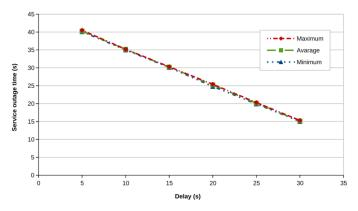
Fig. 3. Service outage times in the function of the delay from the last **OSPF Hello Message** to the stopping of the R2 router
