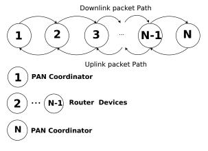
Fig. 2: LWSN Topology and type of network devices
