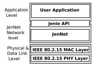
Fig. 3: Detailed Software and Network Stack for LWSN node
