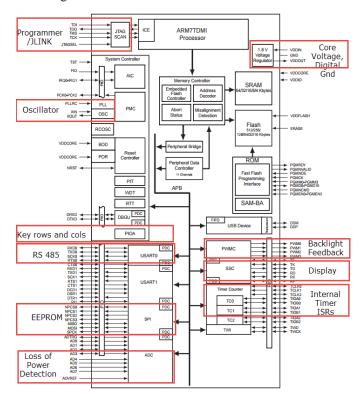
Fig. 3. AT91SAM7S Block Diagram and Pheripherals Used
