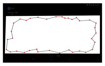
Fig. 10: A screenshot (Tablet with Android operating system) containing a projection of the skew polygon into two dimensions: each two consecutive red points represent a side of the polygon. Note that, at the closing point of the polygon, we have a relatively long segment, which is due to cumulating errors of the sensors.
