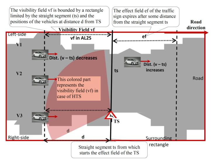
Fig. 7: TS as a plan. The road and a TS projected into a two dimensions space. The road is colored in grey, the vf of the HTS is colored in orange and vf of the soft TS (in AL-S<sup>2</sup>m) is indicated by a discontinuous arrow.
