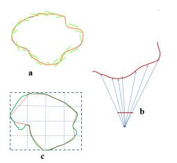
Fig. 1: Implicit surface representations : a. Marching cube, b. Ray tracing, c. Point based method
