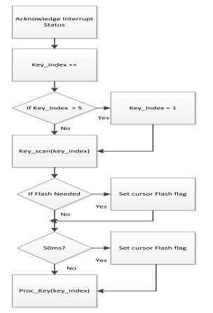
Fig. 7. Timer 1 (1ms) – Interrupt Service Routine
