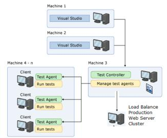
Fig. 4. Load Test Architecture
