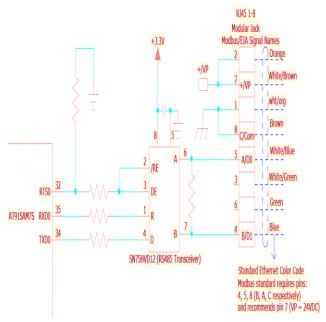
Fig. 17. Schematic of the RS485 circuit
