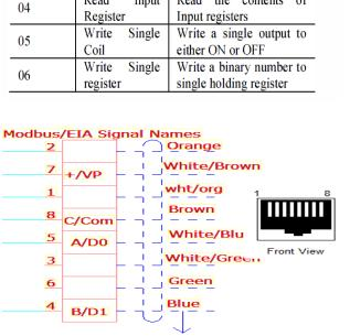
Standard Ethernet Color Code Modbus standard requires pins: 4, 5, 8 (B, A, C respectively) and recommends pin 7 (VP ~ 24VDC)
