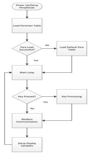
Fig. 6. Operator Panel Interface Main Call Graph
