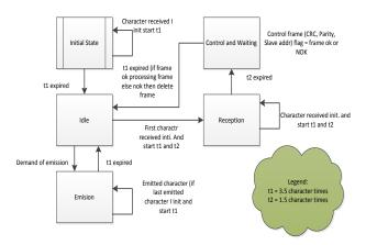
Fig. 11. Modbus Master Transmission Mode State Diagram
