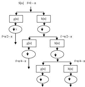
Fig. 1. The decomposition process of DWT at second level
