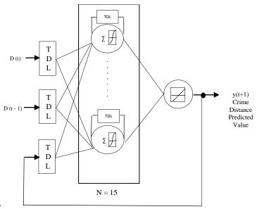
Fig. 4. Nonlinear autoregressive NARX model with exogenous inputs
