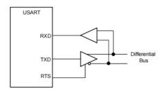
Fig. 2. Connection to a RS485 Interface
