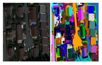
Fig. 3: Example of segmentation result using Statistical Region Merging (SRM) method. From left to right: Original image and its SRM segmentation result.
