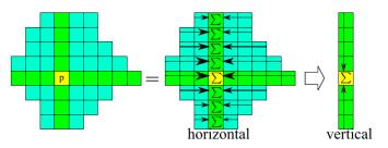
Fig. 1: Calculation of the average likeliness using cross-based aggregation (Mei *et al.*, 2011 [5]).
