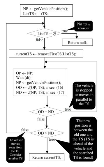
Fig. 8: Seeking the first TS. The symbols used in the diagram are well known (rectangle: processing; lozenge: testing; arrow: control flow). However, we added a bullet symbol for comments.
