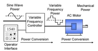
Fig. 1. High level illustration of a Variable Frequency Drive (VFD)
