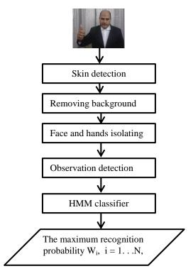
Fig. 2. Proposed system architecture
