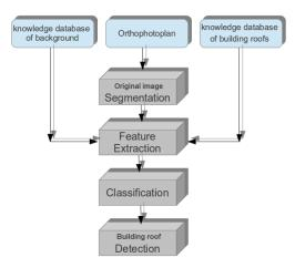
Fig. 2: General flowchart of the proposed building-detection method.
