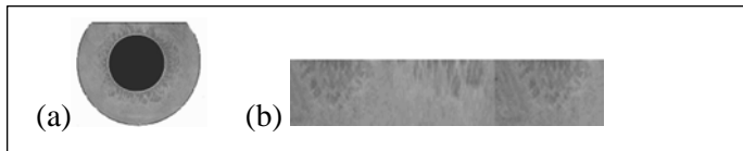
Fig. 6. Example of iris normalization: (a) The iris localized area. (b) The normalized iris area
