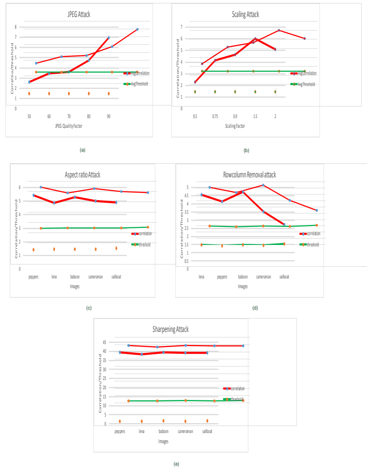
Fig. 1. Robustness of Proposed Technique against different types of attacks. (a) Comparison of average correlation values of five standard images after JPEG compression attack with quality factors changes from 50 to 90, against dynamic threshold. (b) Comparison of average correlation values of five standard images after scaling attack of different scaling factors i-e from 0.5 to 2, against dynamic threshold. (c) Aspect ratio attack of 2:7 in relation to x and y axis. (d) Row Column removal attack (17, 5). (e) Sharpening attack
