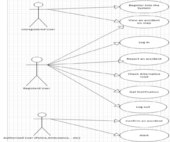
Fig. 5. The designed System boundary for Emergency Services
