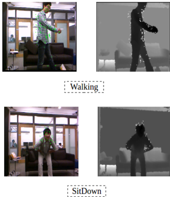
Fig. 6. Motion points in RGB and depth frames of different action represented by green points on RGB frame and white points on depth frames.
