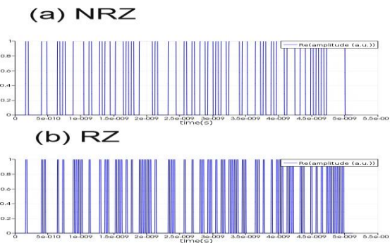
Fig. 2. NRZ & RZ Oscilloscope analysis
