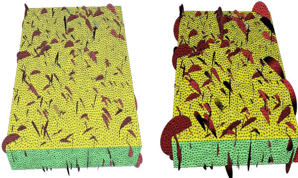
Fig. 9. (a) 3D optimized fracture map and (b) initial 3D fracture map generated in first realization
