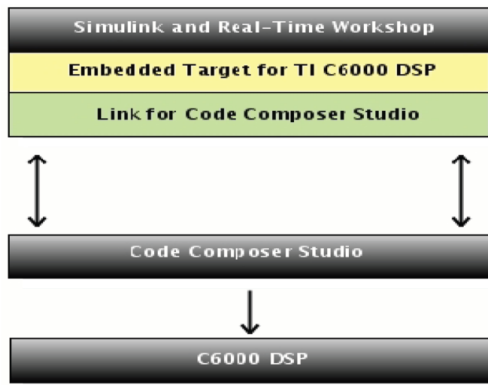
Fig. 8. Flow Diagram connecting Simulink and Real Time Workshop with DSK C6416
