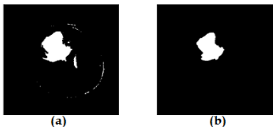
Fig. 9. The resultant display image of morphology step, (a) the result of order static filter showing in 7 (b), (b) the resultant image after applying morphology
