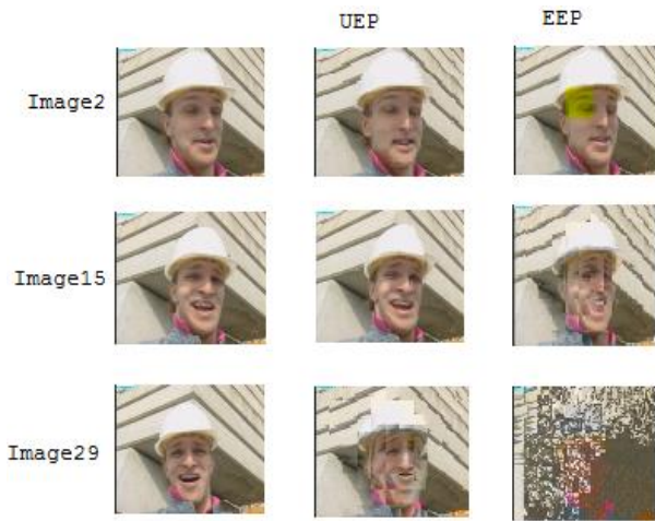
Fig. 9. Images taken from Foreman sequence (left), images encoded by this unequal error protection UEP (middle), and image encoded by equal error protection EEP (right)
