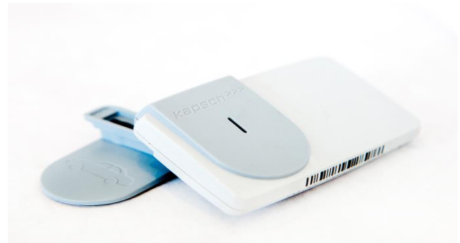
Fig. 4. Example of active tags used for payment on highway
