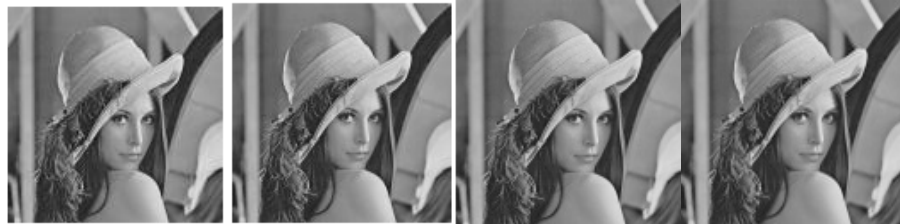
(a) 34.28 dB for Q=75(b) 36.99 dB for Q=85(c) 43.53 dB for Q=95(d) 36.98 dB for Q=95 (Arch.Deg3) (Arch.Deg3) (Arch.Deg3) (Conventional CLDCT)
