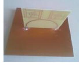
Fig. 13. Realized metamaterial antenna.
