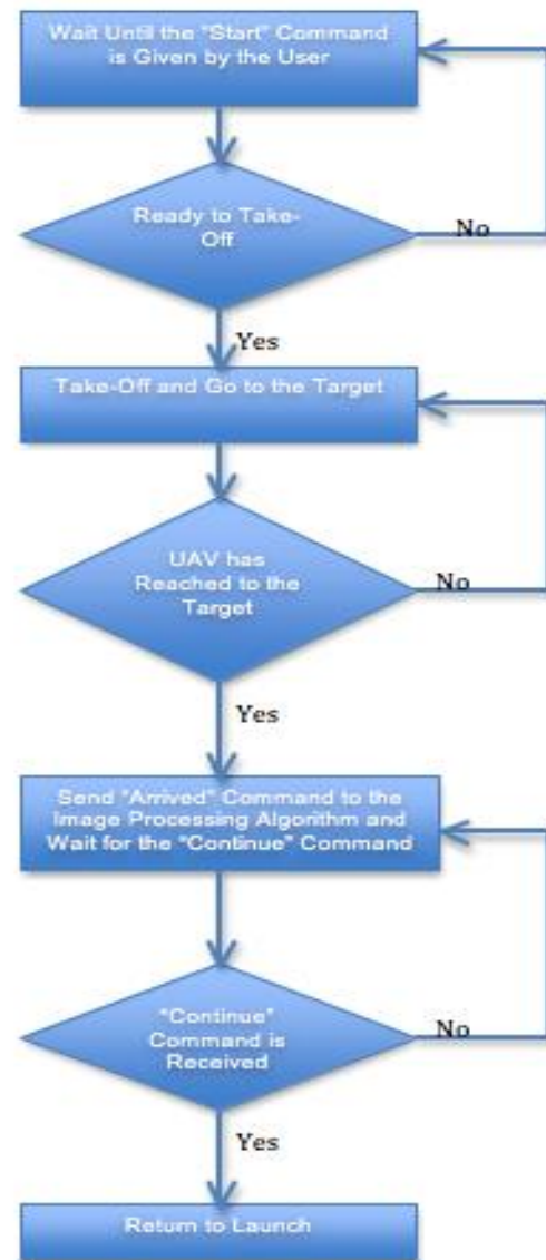
Fig. 3. The Algorithm of Autonomous Flight Software.
