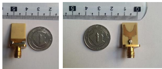
Fig. 5. Fabricated prototype of the antenna (top and bottom view).
