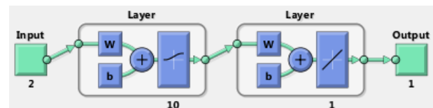
Fig. 6. Structure of designed MLPFFNN.
