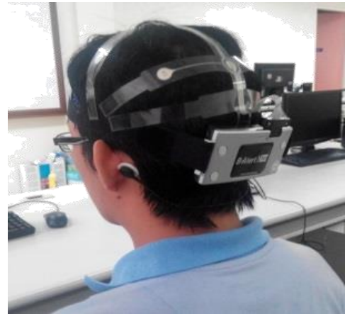
Fig. 1. The medical-grade 9-channel EEG acquisition device is shown being worn by a participant in the study.
