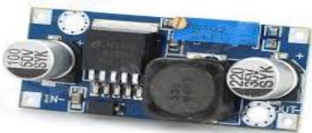
Fig. 10. Voltage step down regulator.
