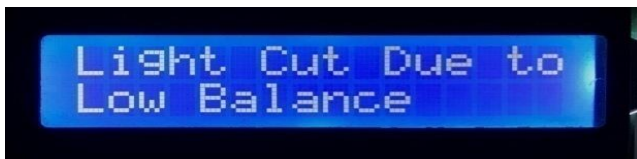
Fig. 9. When energy meter cut off the load due to insufficient balance.
