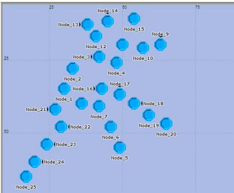
Fig. 12. OPNET generated 25 nodes WMN topology.
