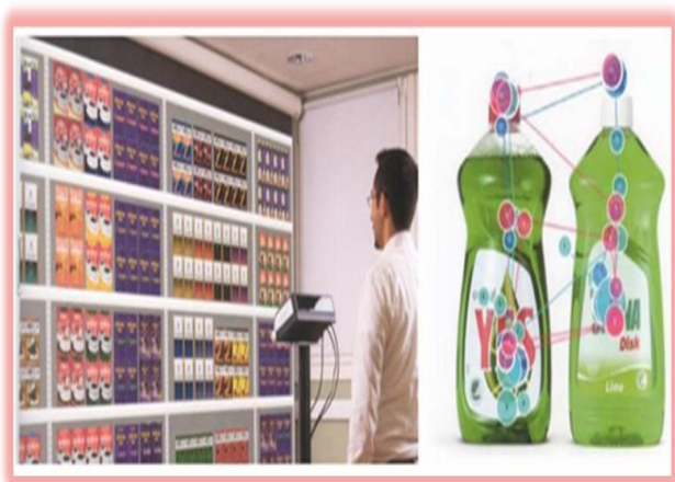
Fig. 16. Customer gazing upon a product, points of visual attention marked by the eye tracker
